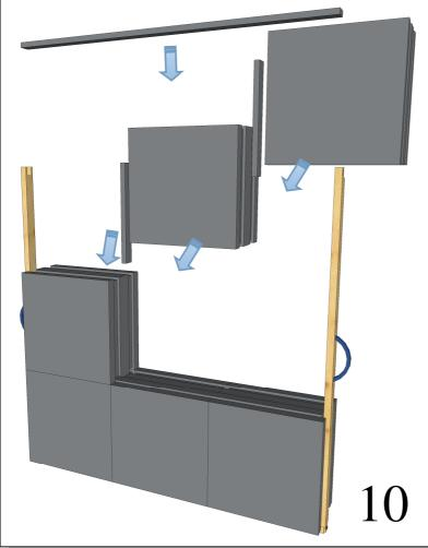
10. Now the frame is filled with the rest of the foam modules. The modules are mounted in the same way as the first row, as shown to the left.
