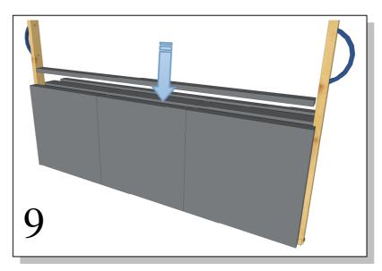
9. The one long infill part is mounted at the top and is pushed down into the front groove.
