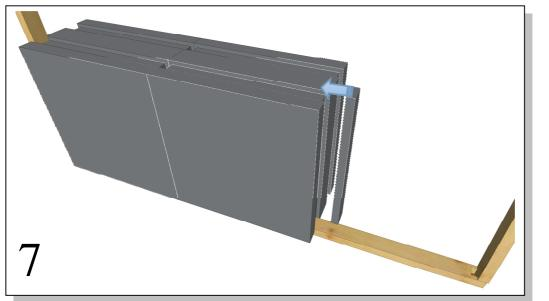
7. Another short infill part is mounted in the groove to the right of foam module no.2. Remember that the infill parts must be mounted only in the front grooves.
